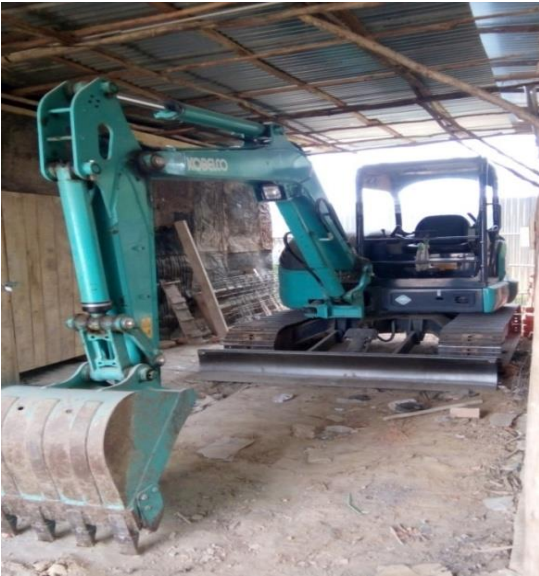
Gambar 10. Excavator Bakchoe roda kelabang
