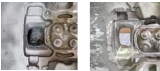
Gambar 4. Improvement Gate , (a) Before Improvement , (b) After Improvement
